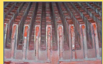
The NitroJet successfully removed winding materials from a burned-out motor at the Brown's Ferry power plant. Left photo: motor before cleaning; Right photo: motor cleaning in process.
