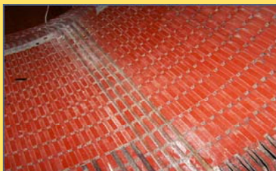
The NitroJet successfully removed winding materials from a burned-out motor at the Brown's Ferry power plant. Left photo: motor before cleaning; Right photo: motor cleaning in process.
