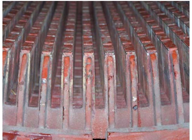
Stator after removal of motor windings.
